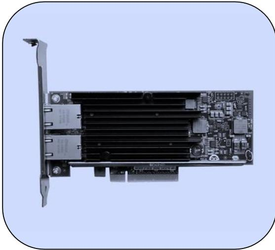
10GBASE-T converged network adapter simplifies migration to 10GbE, provides iSCSI, FCoE, Virtualization, and Flexible Port Partitioning.
