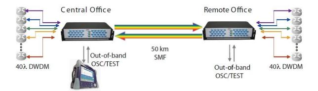
Point to point link with Optical Monitoring
