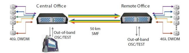
Point to point link with Optical Monitoring
