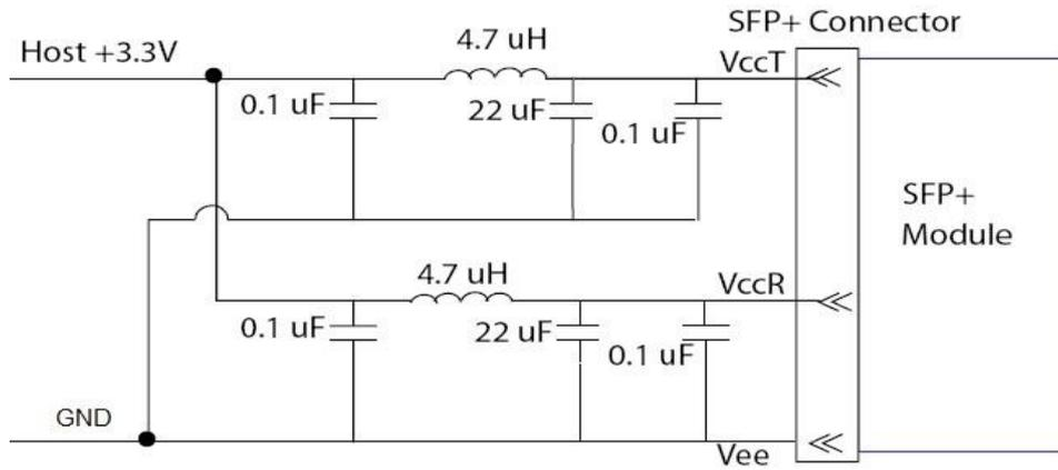
Figure 3. Host Board Power Supply Filters Circuit
