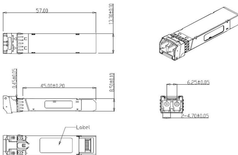
Figure 5. Mechanical Specifications
