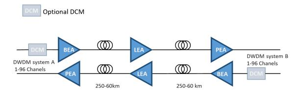
**X8600-20G17(V)** is a single stage EDFA Amplifier typically used as booster amplifier (BEA) for amplifying transmission signals ether single channel or multiplexed multichannel. Saturated output optical power is 20dBm.
