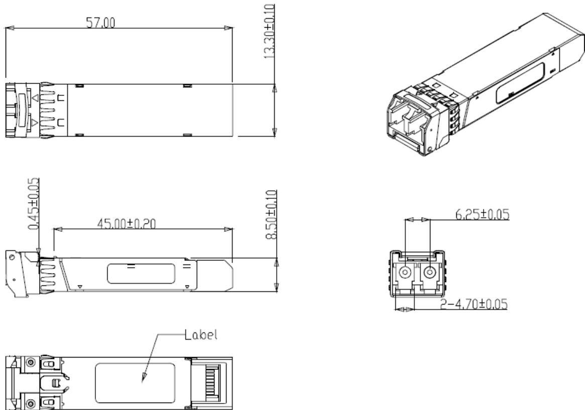
Figure 5. Mechanical Specifications
